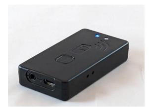
The device is essentially an APRS modem with a KISS TNC built in and Bluetooth connectivity. The device charges via USB-C. Mobilinkd provides a configuration app for your mobile device that allows you to set internal packet parameters. Typically, this needs to be done once for your target radio and then never again. Mobilinkd also sells adapter cables to go from the TRRS jack on the device to your radio's external mic and speaker jacks. Nearly all of the common HT manufacturers are supported.
